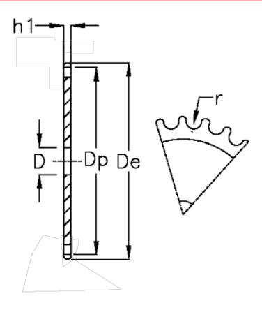
C = 4 D = 30 De = 646 Dp = 631.01 For chain size = 1 1/2 x 1 For chain type = 24 B-1 h1 = 24.1 Sumber of teeth = 52
